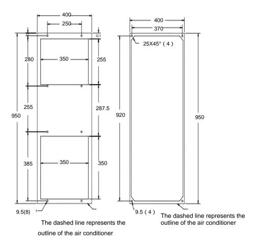
Wall mounted installation hole diagram
