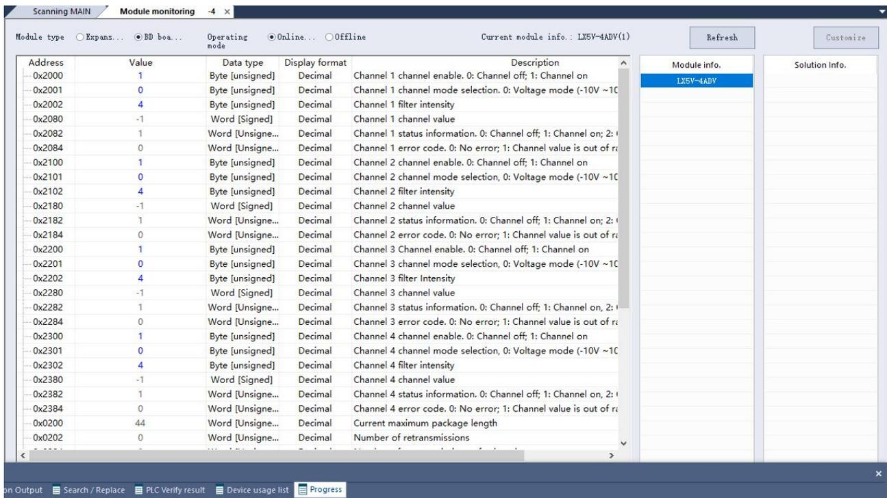
① 4ADV buffer memory (BFM): Used for 4ADV-BD module status monitoring.
