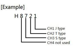
The time of A/D conversion is 240ms for each channel. When "3" (unused) is set for a channel, this channel would not have A/D conversion, therefore, the total time for conversion decreases. In the above example, the conversion time is as follows:
