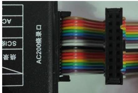
The burn-in cable is plugged into the "AC300 burn-in port"
