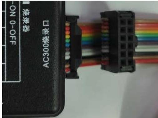
The burn-in cable is plugged into the "AC300 burn-in port"
