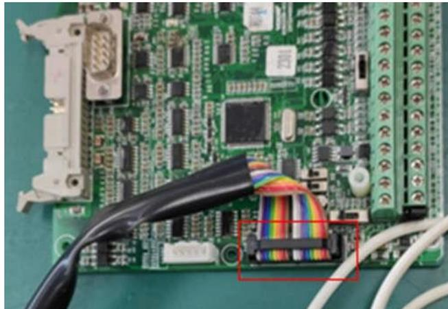
The burn-in cable is plugged into the expansion port of the AC80CCON control board
