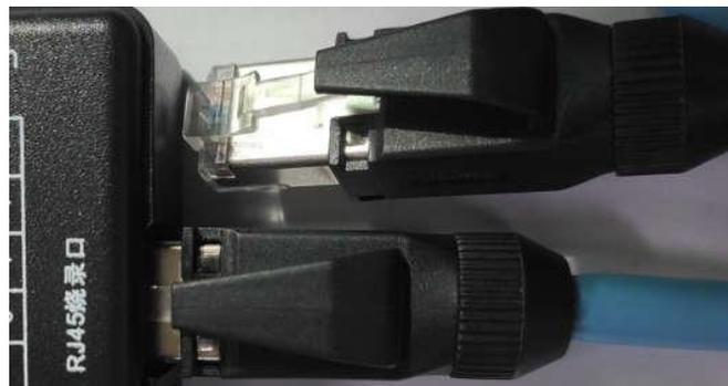
The burn-in cable is inserted into the "RJ45 burn-in port"
