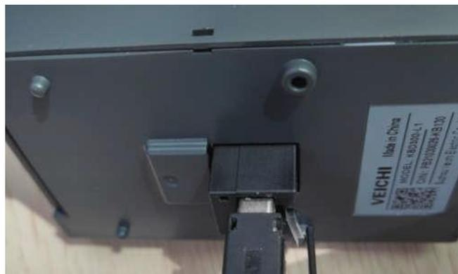
Insert the network cable of the burn-in port into the keyboard
