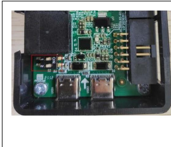
When USB1 is damaged, open the top cover of the controller and turn the internal black dip switch to ON.USB2 can be used as a backup burn-in port.The function is the same as USB1.
