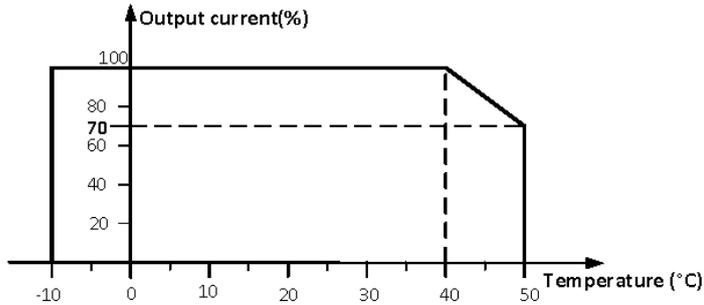
Chart 3-2:AC10 series drive derating curve while over permit temperature
