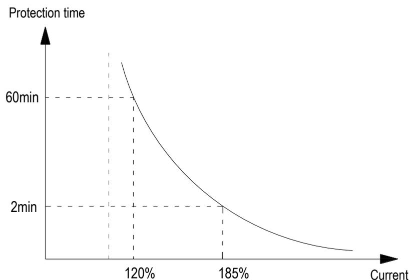
In the above figure, the horizontal axis is the current entering the protection curve, that is, the percentage of the rated current of the motor. The calculation formula is: horizontal axis current = (motor actual current / motor overload protection coefficient) × 100%, so increasing
