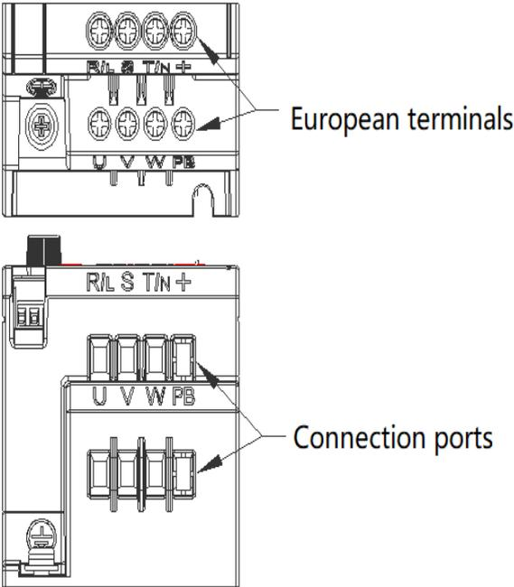
0.4kW-5.5kW Terminal arrangement
