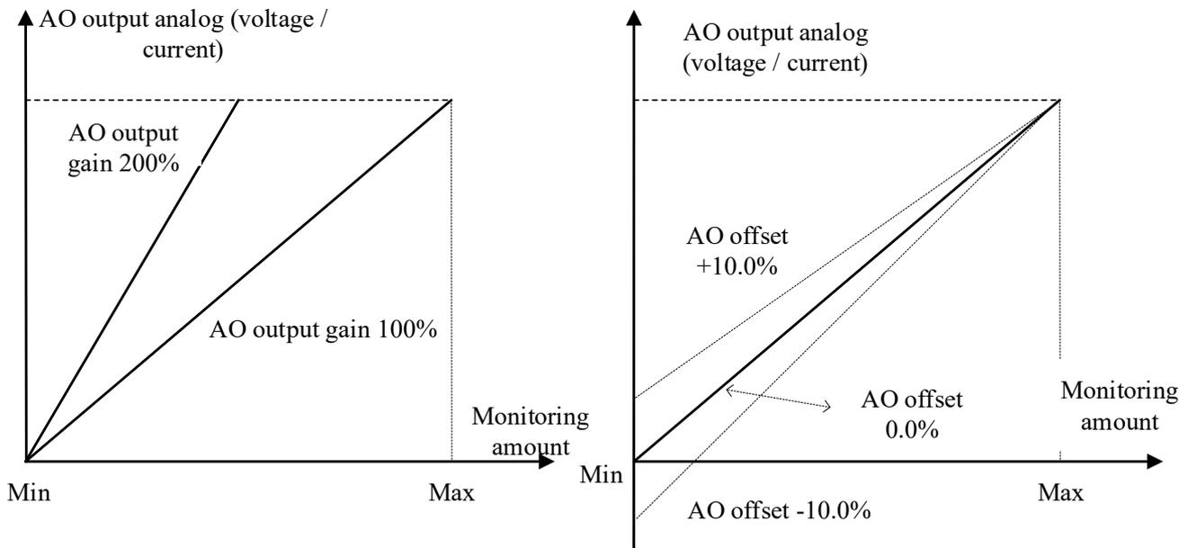
AO analog output and gain, offset schematic
