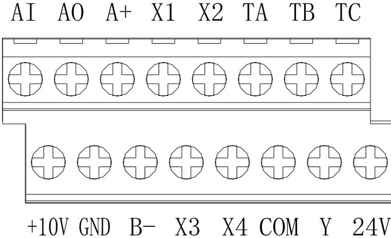
7.5kW-22kW Control circuit terminal arrangement
