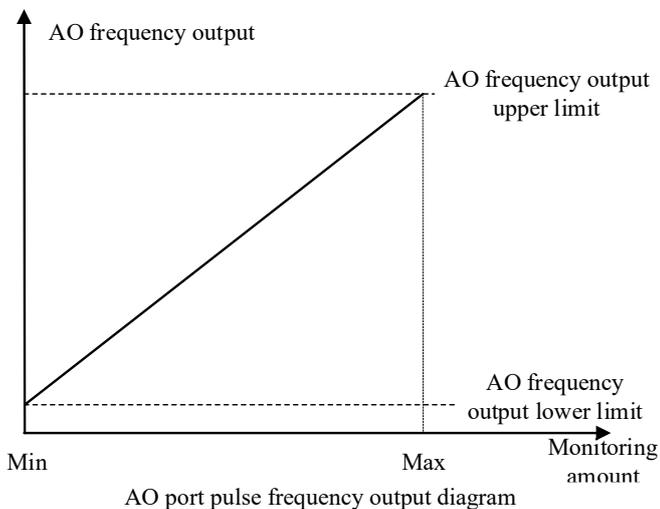
AO port pulse frequency output diagram
