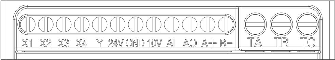
0.4kW-5.5kW Control circuit terminal arrangement
