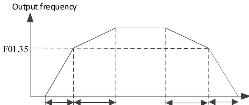
Output freq.  $\geq$ F01.35 is added and Dec. according to F01.22 & F01.23 [addition and Dec. time 1]
