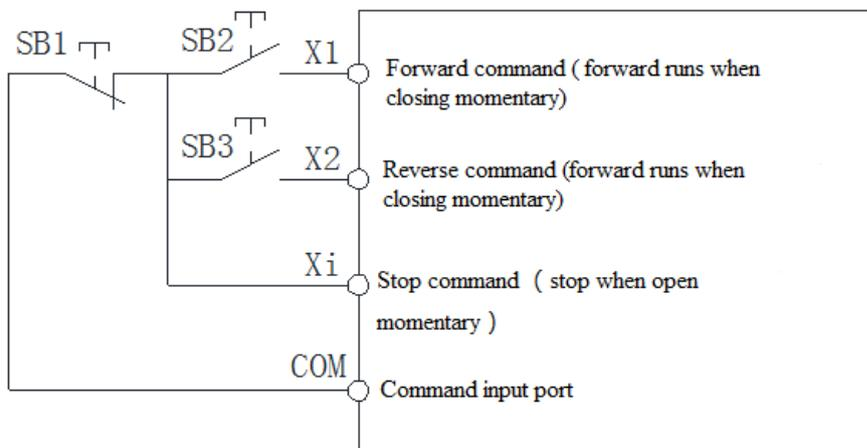
Hint: SB1: Stop button; SB2: Forward run button; SB3: Reverse run button; "Xi" is multi-function input terminal set to "3" [3-wire operation control (Xi)].
