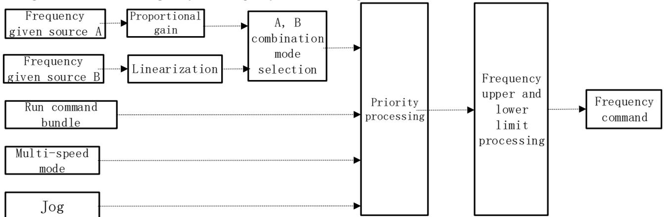
Frequency command given schematic
